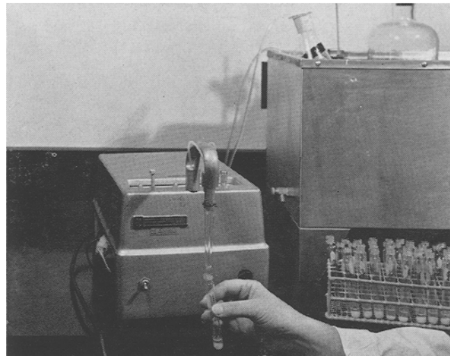
FIG. 2. Mechanical pipetting unit (b) for pipetting petroleum ether and water.
