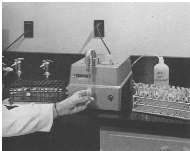
FIG. 1. Mechanical pipetting unit (a) for pipetting serum and alcoholic potassium hydroxide.
